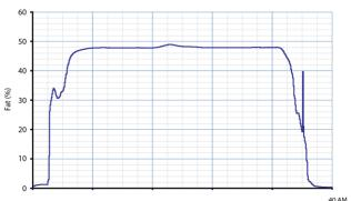
Continuous in-line monitoring of extra thick double cream.
