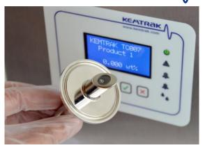
Traditional turbidity based optical measurement instruments lack resolution and are not reliable at concentrations above 1% suspended solids due to the high optical density of the process media. This limitation is overcome with the <a href="Kemtrak TC007">Kemtrak TC007</a> and for the first time the operator can monitor and have complete control over their dairy process at any concentration.
